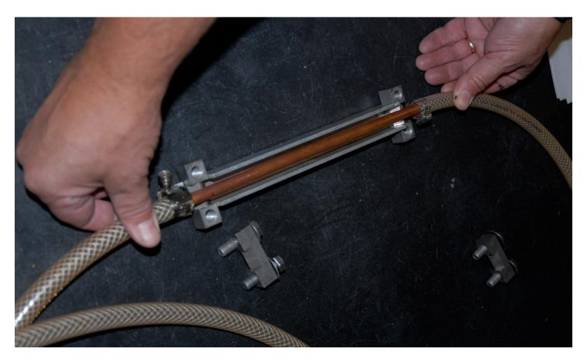
Insert the copper tube into the plastic hose about 2 cm and secure using the hose clamps as shown.
