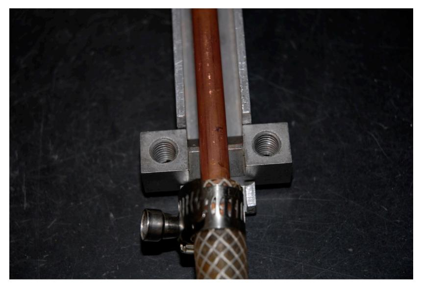
Replace the upper portion of the pinch clamps and tighten using fingers only (do not yet deform the copper tube by excessive tightening).
