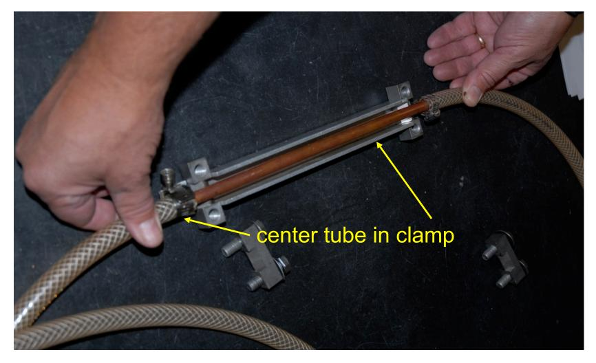
• Centering the copper tube in the clamp is very important.
